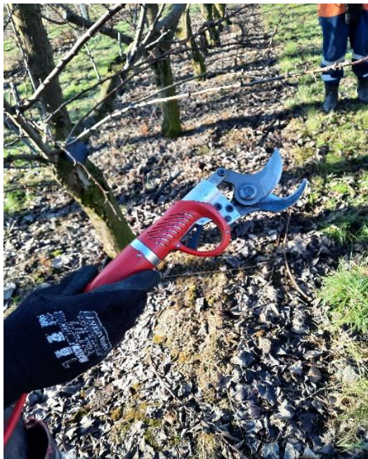
Figure 5.4: Electric secateurs for pruning fruit trees. They require less force to create the cut
